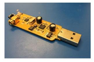
An RTL-SDR "dongle" for software defined radio. Allows any computer to receive radio signals through a usb port. They are available for under \$20 and excellent for use in high school science projects.
