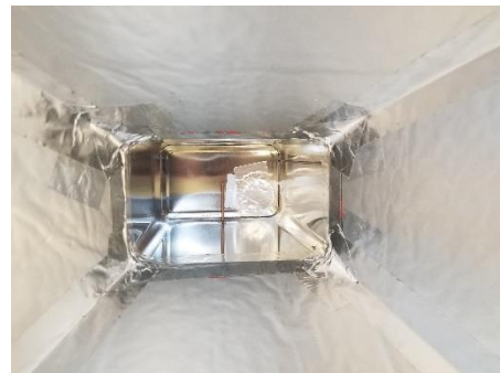
Looking down into the can from the mouth of the horn. Notice the taping along the corner edges and at the can/horn seams.
