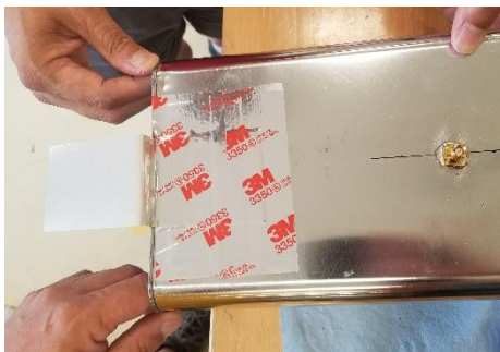
Flashing piece taped to can.
