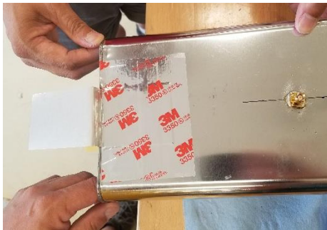
Flashing piece taped to can.
