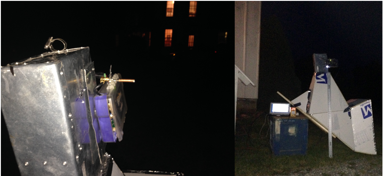
FIGURE 2: AT LEFT, FEED PROBE AND HORN POINTED TOWARDS THE TEST SIGNAL SOURCE. AT RIGHT, WAVEGUIDE MOUNTED ON FOLDED HORN, SIDE VIEW. THE 48IN RULER, LEANING ON THE HORN, SHOWS THE SCALE OF THE SYSTEM. THE COMPUTER AND POWER SUPPLY ARE BEHIND THE HORN.
