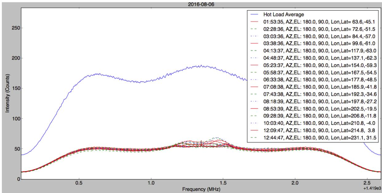
Figure 4: Plot of half hour averages of uncalibrated intensities versus frequency (MHz) on August 6, 2016. The top most plot is the average of all data when the horn was pointed at the ground. The red and other dashed curves show the variation with position on the sky.
