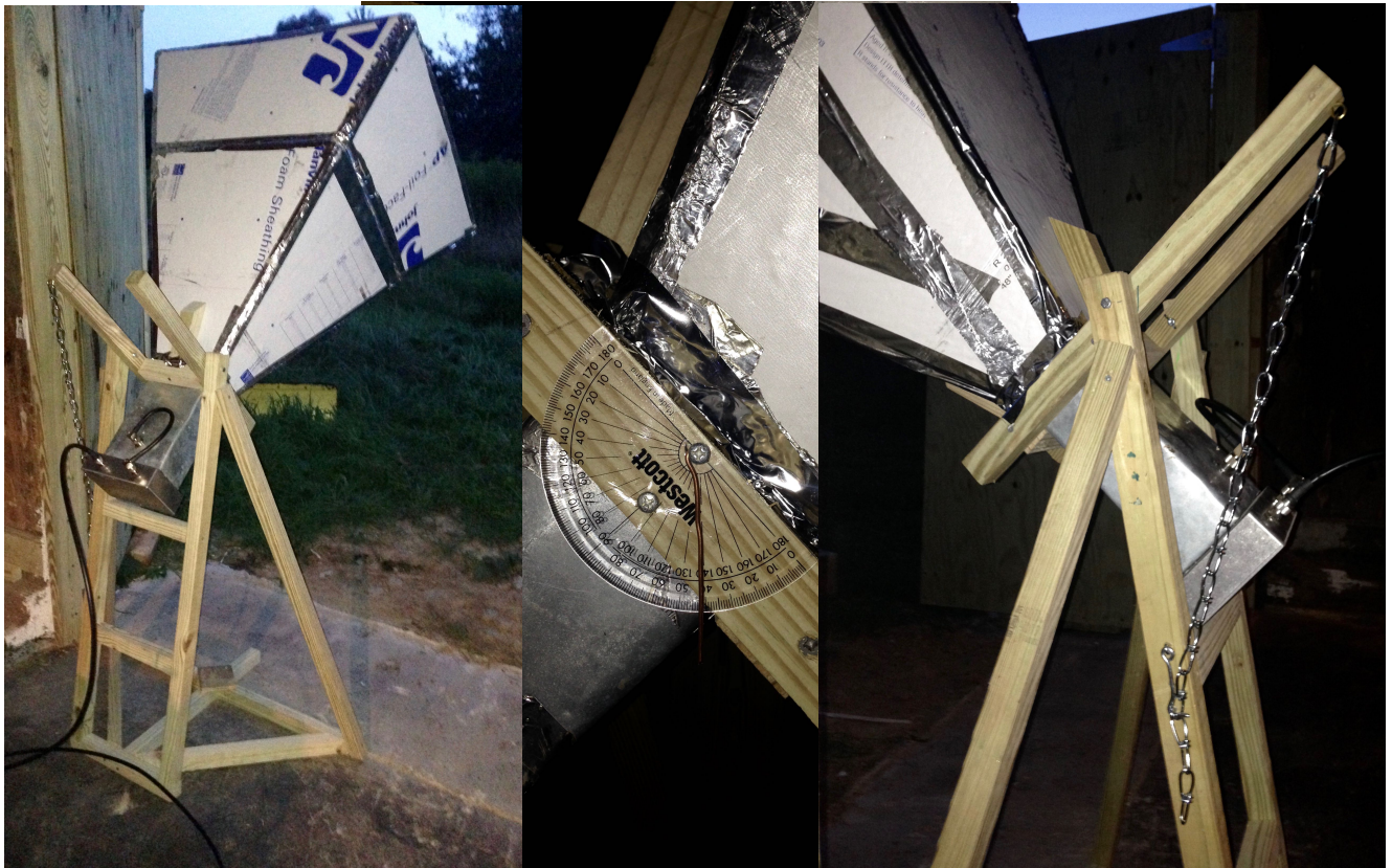
Figure 1: Images of the Horn you can Build and use to map the Milky Way. The image at left shows the exterior of the horn, which is a 4 sided pyramid, with large, open end pointed at the sky. The opening is a 36x32 inch rectangle. The horn is constructed of aluminumized foam insulation, held together with aluminum tape. The lower end feeds a 4x8 inch wave guide. The waveguide is constructed from a riveted aluminum sheet. The image at center shows the gauge used to read the horn elevation. The image at right shows the hook and eye mechanism for locking the horn at a specific elevation. The chain links had a spacing that corresponds to between 5 and 10 degree steps in elevation. Since the horn has a 13 degree full width at half maximum resolution, the chain links provided sufficiently small steps to cover the entire sky.
