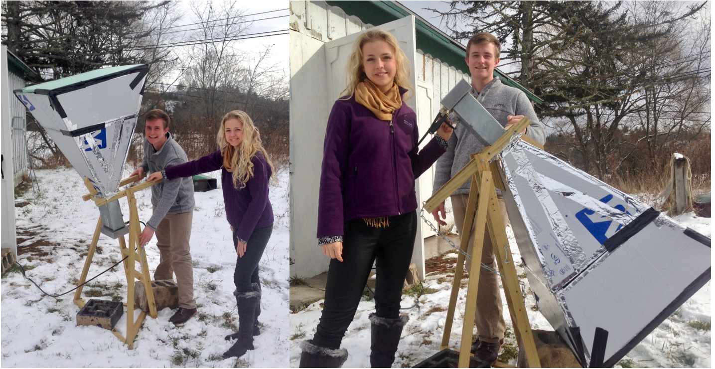
Figure 2: At left, Nathaniel and Regina are setting the horn elevation for an observation. Next they start the computer collecting spectra. After a 24 hour period of observations, the data are calibrated by a half hour observation of the ground. At right, Regina and Nathaniel have just started a calibration observation. The weather was cold but clear for their observations. Note in the left image, a sheet of green foam insulation covers the horn to allow observations in bad weather. This foam is very transparent to radio waves. However data taken during the snow storm were not usable, due to snow piling up on the top of the horn.
