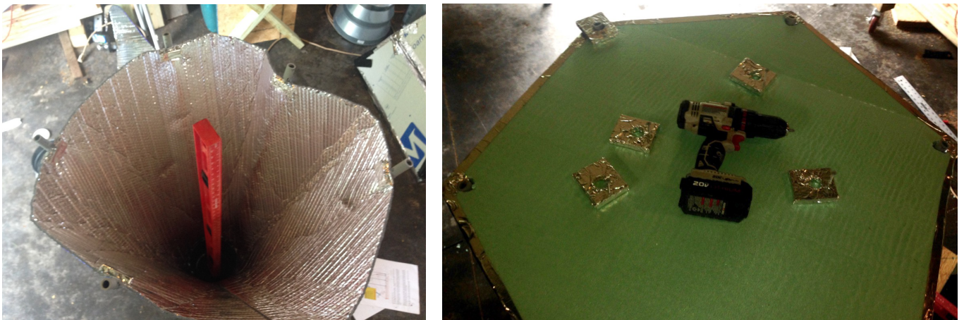
Figure 12: Horn attached to reducer, but no cap yet. At right the horn lid is being attached to the legs. Because of the symmetry of the horn, the lid can act as a table, for light weight items.
