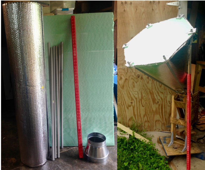
Figure 2: Large Parts of Cone Horn (Left). The Bubble Wrap and green foam board are 4-feet tall. The cone legs are 39-inches long segments of grey conduit. The red ruler is 4 feet long. The galvanized 6-inch to 8-inch pipe reducer is by the ruler.
