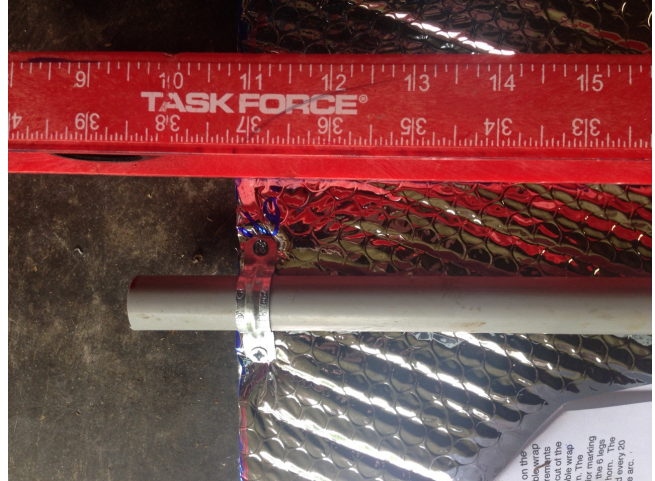
Figure 8: Steps of cutting wrap and attaching pipe legs. The upper left figure shows drawing the inner and outer arcs, the 1.5-2-inch overlap on both sides and measuring and marking the leg positions. Starting with the center pole, add the inner piece of the lid plywood part.
