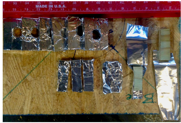
Figure 6: Steps for making attachments for legs and end caps to hold lid on. The upper left shows steps for making the 6 end caps. These are made two at a time by placing two lengths of 2.5-inch wide plywood strips on top of each other. Mark the strips every 3 inches, then draw a center line. At 1/4-inch from each edge and 1 1/4-inch mark spots for drilling with 1/8 inch drill bit.
