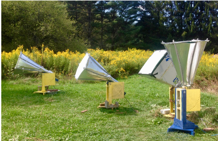
Figure 1: Four radio telescope horns all simultaneously observing different elevations on the sky. These horns each have an aperture area of roughly 0.5 \text{ m}^2
