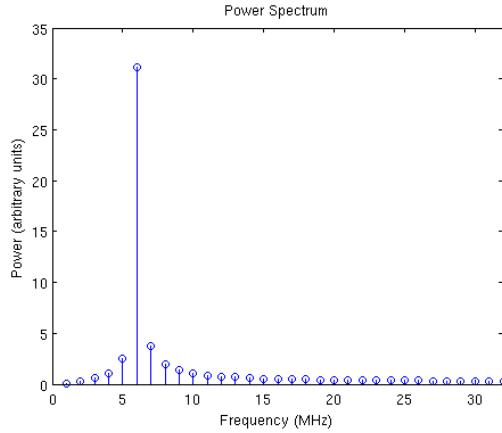
A 5.1 MHz tone convolved with a sinc function leads to spectral leakage<sup>12</sup>
