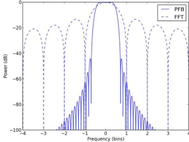
In GnuRadio, the variables associated with the Polyphase Filtering define the sinc function shape. The delay blocks serve to split the stream into four consecutive chunks, each with a number of samples equal to the number of bins in the FFT. The multiplication by the correct part of the sinc function is made, and the results added together like in the diagram at the top of the page.
