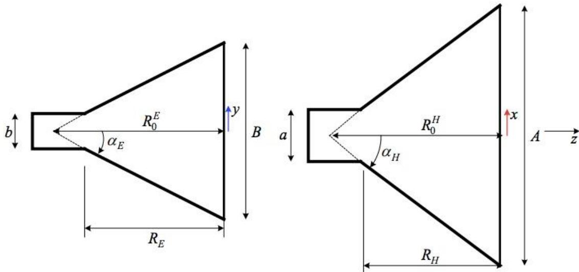
We take  $A=75.4$  cm (just able to fit through a 30" door), and from above  $a=16.8$  cm and  $b=10.5$  cm. For an optimal pyramidal horn, we can calculate  $B=59.7$  cm (The DSPIRA horn is 60.1 cm, which is almost identical and likely due to using imperial units) using
