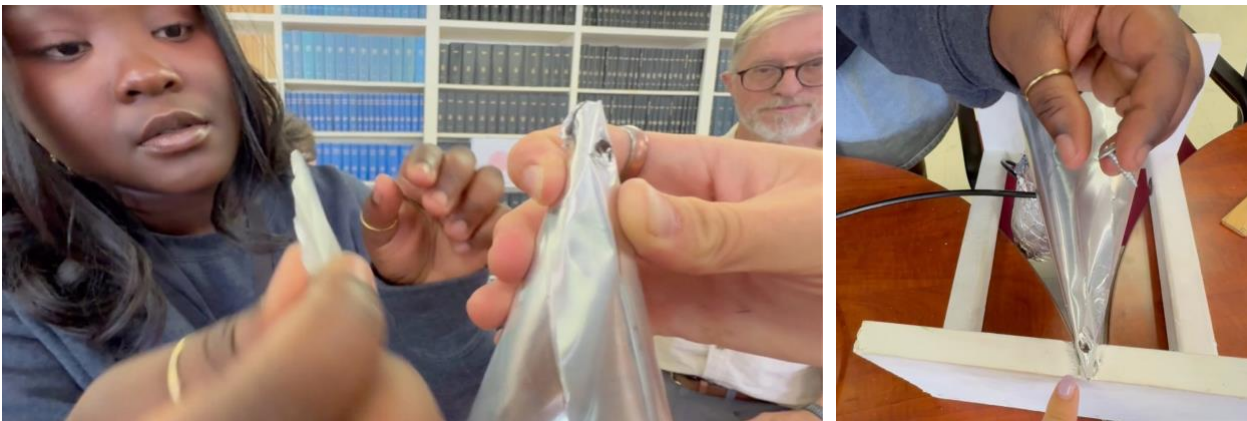
Fig 10: Nana, Austin and Glen secure the pointed end of the cone and protect us from sharp edges of the flashing (left). Nana screws the point of the cone to the back of the elevation mount with a 1.25-inch-long wood screw (right).
