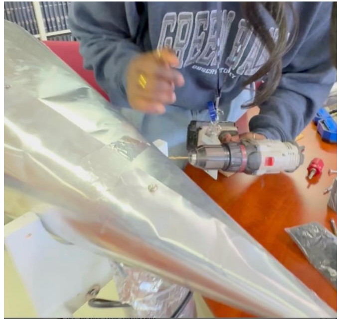
Fig 11: Nana drills through the sides of the wooden front part of the elevation mount. After drilling, we attach the cone-horn to the elevation mount from the inside, with two 1.25-inch-long wood screws.
