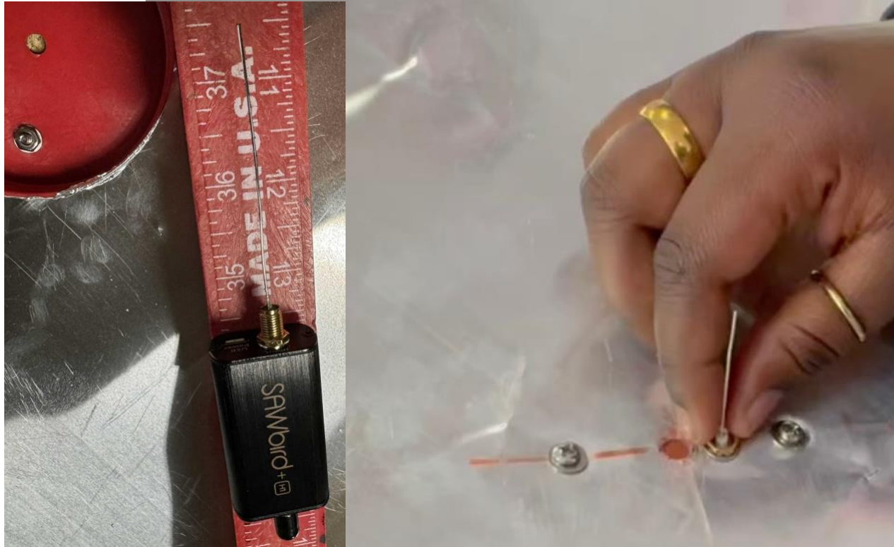
Fig 7: The feed probe can be separate from the amplifier or directly soldered into the input of the amplifier (left). We found the telescope was more sensitive and reliable if the probe was soldered into the amplifier. Cut the feed probe to length, 1.73 inches. Add metal tape to make the transition from the flashing to probe smooth.
