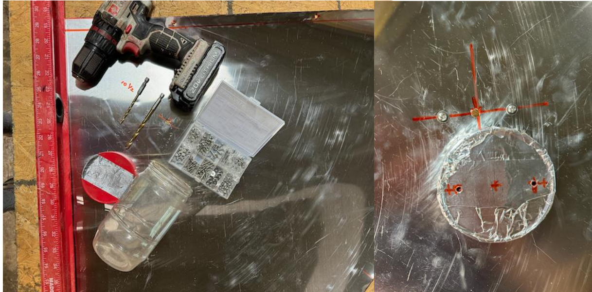
Fig 5: After cutting the semi-circle of flashing, the next step is drilling the holes for the feed probe and the screws holding the lid in place (left). The feed probe hole should be 10.5-inches from the corner of the semi-circle. After drilling the feed probe, drill two holes either side of the probe hole, spaced by 1.25-inches along the line. Then place the screws and washers in the mounting holes. Place the lid on the other side of the flashing and bolt in place (right).
