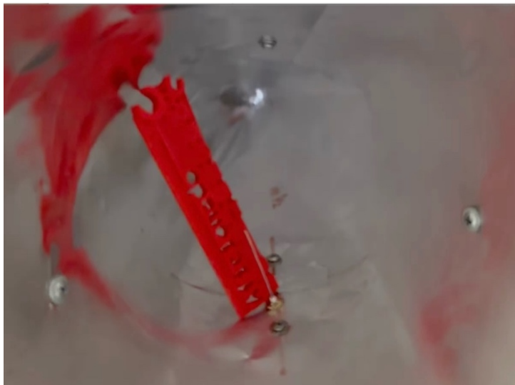
Fig 12: The assembled cone-horn opening, showing the feed probe in front of a short red ruler (left). The feed probe is 10.5-inches from the point of the cone. At right, we zoom in on the feed probe, which is the thin silver wire. The heads of the wood screws for attaching the cone to the mount are visible on the sides.
