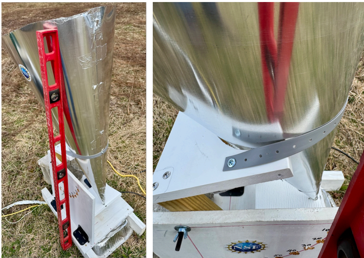
Fig 13: Completed telescope, built from 40in flashing (left). This horn is a little bigger due to finding a source for larger flashing. The red ruler is 4ft tall, for scale. Bigger is better, except in the wind! It needs the pipe strap to hold the horn in place. The strapping is attached by two large head Phillips Screws. The image at right is a zoom in on the strap attachment. One screw on each side is sufficient. I did add a machine screw through the strapping in the middle to hold the horn to the strap. Not sure if that is needed. Tape might be sufficient.
