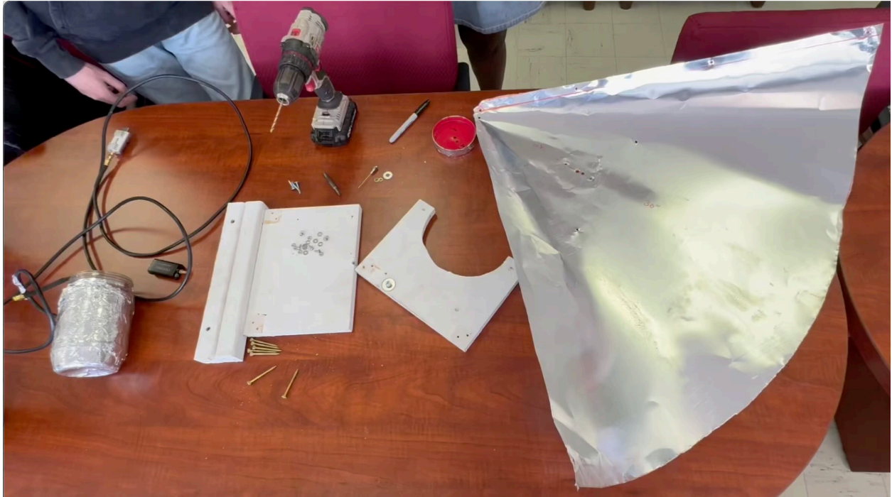
Fig 3: All the parts need to build the cone-horn radio telescope. The biggest piece is the aluminum flashing (right). The wooden parts of the mount are painted white (middle). The mount is held together with wood screws. At left are the LNA, metal tape covered peanut butter jar, high-quality coaxial cable (LMR 240) attached to the AIRSPY-Mini SDR. The feed probe and metal screws are at the top middle.
