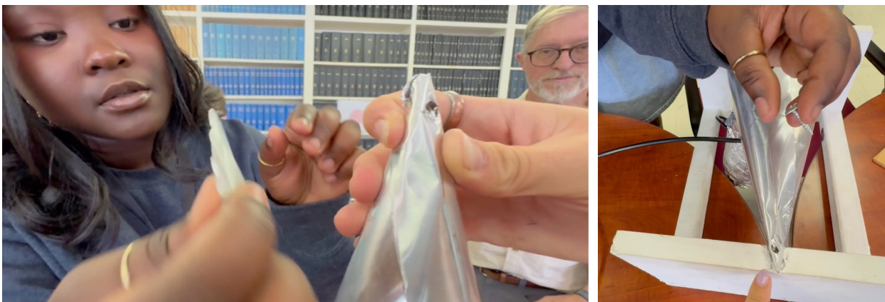
Fig 10: Nana, Austin and Glen secure the pointed end of the cone and protect us from sharp edges of the flashing (left). Nana screws the point of the cone to the back of the elevation mount with a 1.25-inch-long wood screw (right).
