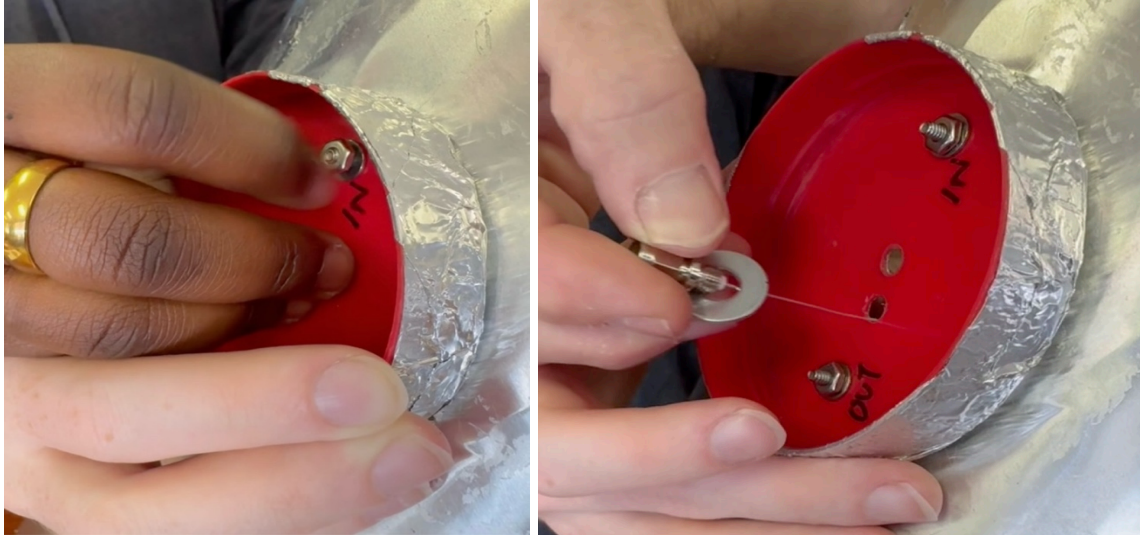
Fig 6: Bolt inside of peanut butter jar lid to the cone (left). Next, insert the feed probe into the horn, where the signals will be received (right). In this picture we'd moved the feed probe position to 10.5-inches, from the original placement.
