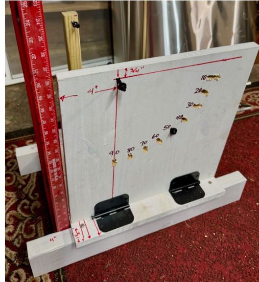
Figure 10: Protractor side of the base, with hinges screwed in place.
