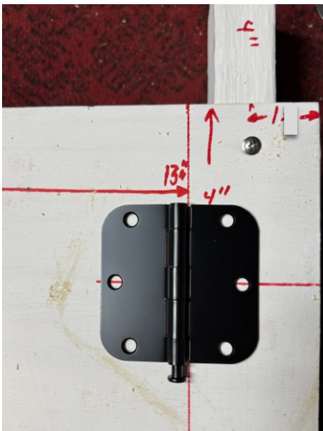
Figure 9: The front hinges are centered 4-inches from the front of the base. Along the center holes. Drill and attach with screws to the left side of hinge.
