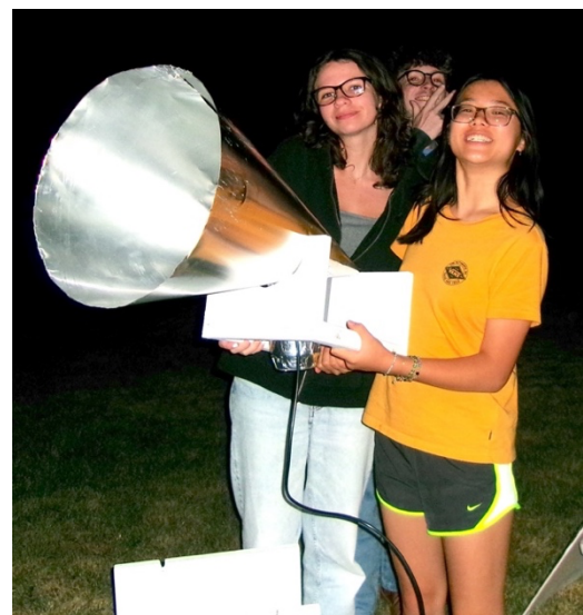
2024 Green Bank Summer students Kait, Sophia and Austin with Cone Horn Telescope, 30" tall, on elevation mount.
