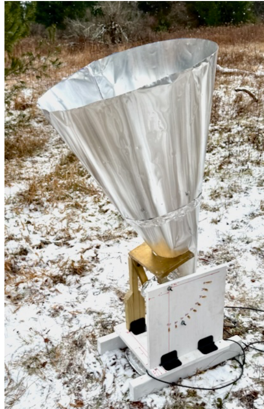
Figure 12: The completed base with double sized cone radio telescope, Because the base is wide and low, it is stable. But it does not hurt to put a concrete block on the base, in case of high wind.
