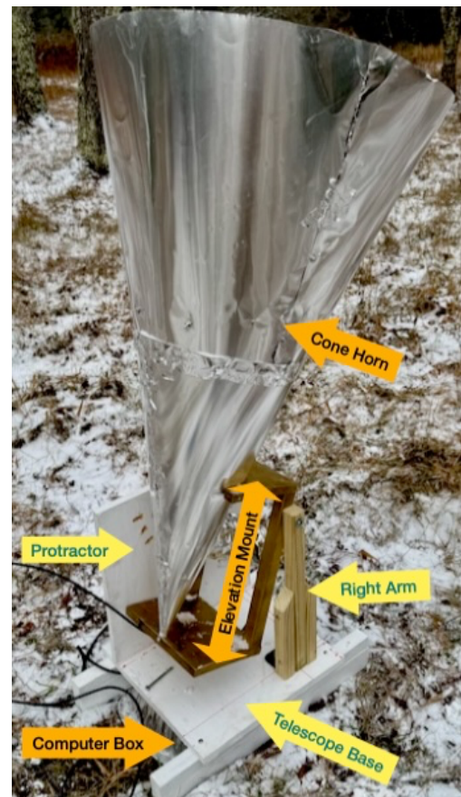
Figure 1: Completed Telescope, marking major parts. Here we describe the Telescope Base (Blue Text). Other memos describe the Cone Horn, Elevation Mount and Computer
