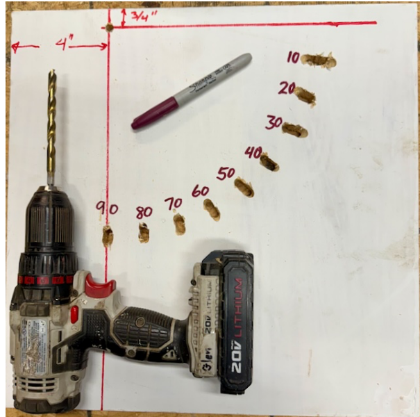
Figure 8: Protractor drilled. Use a permanent marker to add the elevation angles. 90 degrees is at the bottom, for a telescope pointing straight up.
