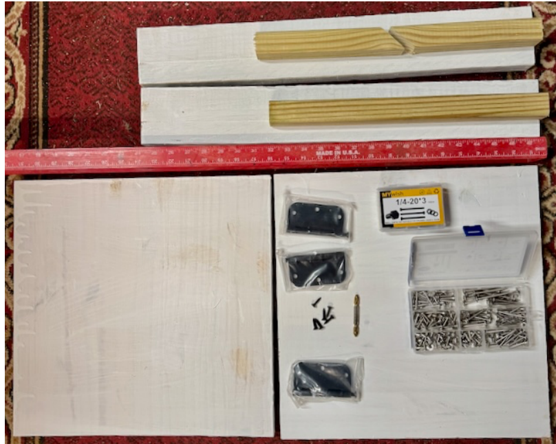
Figure 2: All parts of the telescope base. At the top there are two 2x4s, each 2-feet long and two 16-inch sections of a baluster. One of these two is cut in half diagonally. The red ruler shows the scale. At the bottom are two 16-inch square boards, \frac{3}{4} -inch thick. At bottom right are three door hinges, a box of assorted screws and a box of 3-inch long, \frac{1}{4} -inch thick bolts.
