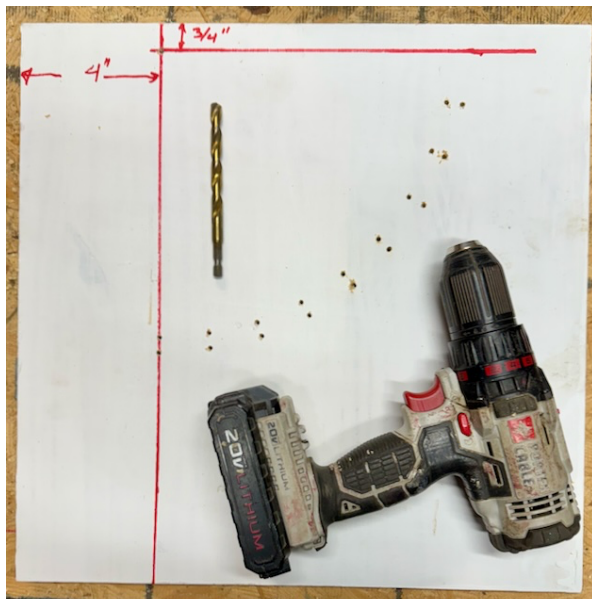
Figure 7: Pilot holes are drilled. Remove the template. Next, take a 3/8-inch drill bit and re-drill each of the pilot holes. The pairs of holes at each angle should connect, by tilting the drill bit along the line towards the top left corner.
