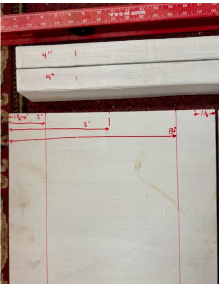
Figure 3: Draw lines +/- 5-inches from the center of the bottom. Mark the leg positions and 4-inches from the ends of the 2x4s.
