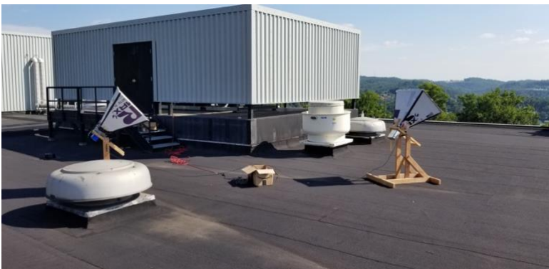
Figure 7: Figure 7 when beam forming, the beam of a single horn is symmetric radially around the horn. However, when we have an interferometer, the beam pattern on the baseline is decreased since we are adding and averaging the beam patterns. Additionally, the beam pattern perpendicular to the baseline remains unchanged. Thus, when wanting to observe the fringes from the sun, one needs to have an east west baseline in order to find the phase difference that comes with beam forming the horns.
