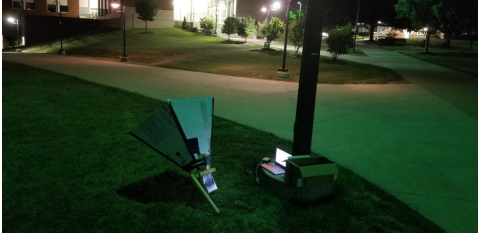
Figure 2: The metal can has 23.7cm height, 16.8cm length, and 10.7cm width as measurements. The antenna was soldered about 5.7 from the bottom of the can and is equidistant from the sides. On top of this can, a trapezoidal horn made from foam was taped to the top of the can to create a collecting apparatus. Aluminum tape was used to connect the can to the horn, which was conductive on the inside, and to seal the sides. The horn has 4.6 square meters of collecting area and is 75.9cm from can to collecting width. The antenna was connected to an SMA connection which transferred the voltage the LNA. The horn itself was set inside of a wooden frame, which was used for long term observing to ensure that the horn remained pointed in one direction.
