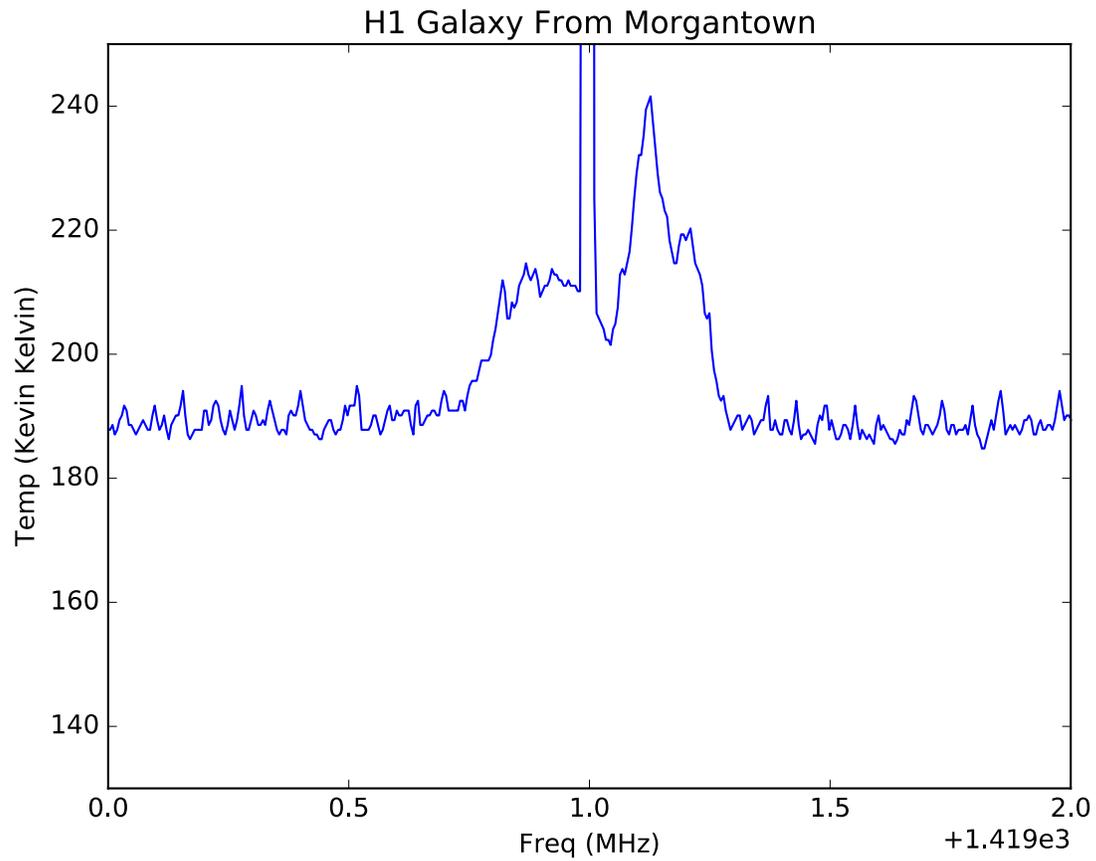
Using an 'on off' pointing at the galaxy, and point at the ground, a rough estimate is made of the system temperature. Looking at the neighboring frequencies, the system temperature was roughly 190K. The galaxy is visible at the center, with the large spike at 1420MHz due to the DC component of the sampler.
