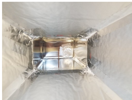
Looking down into the can from the mouth of the horn. Notice the taping along the corner edges and at the can/horn seams.
