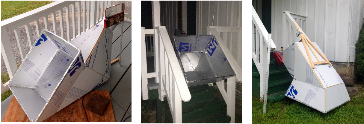
FIGURE 2: WAVEGUIDE FEED HORN AND ELECTRONICS BOX SHOWN IN PROFILE (LEFT), WAVEGUIDE IN POSITION FOR OVERNIGHT ASTRONOMICAL TESTS (CENTER) AND WAVEGUIDE HORN INVERTED FOR CALIBRATION MEASUREMENTS (RIGHT). IN THE LEFT AND RIGHT FIGURES A 48" RULER IS SHOWN TO PROVIDE SCALE.
