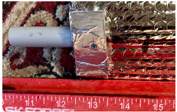
Figure 8: Steps of cutting wrap and attaching pipe legs. The upper left figure shows drawing the inner and outer arcs, the 1.5-2-inch overlap on both sides and measuring and marking the leg positions. Starting with the center pole, add the inner piece of the lid plywood part.
