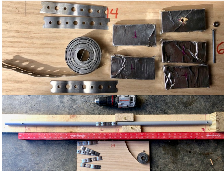
Figure 7: Pipe straps cut to 4 inch lengths for attaching middle of legs to bubble wrap (top). The wooden blocks are wrapped with metallic tape and marked for drilling a 3/16 hole.
