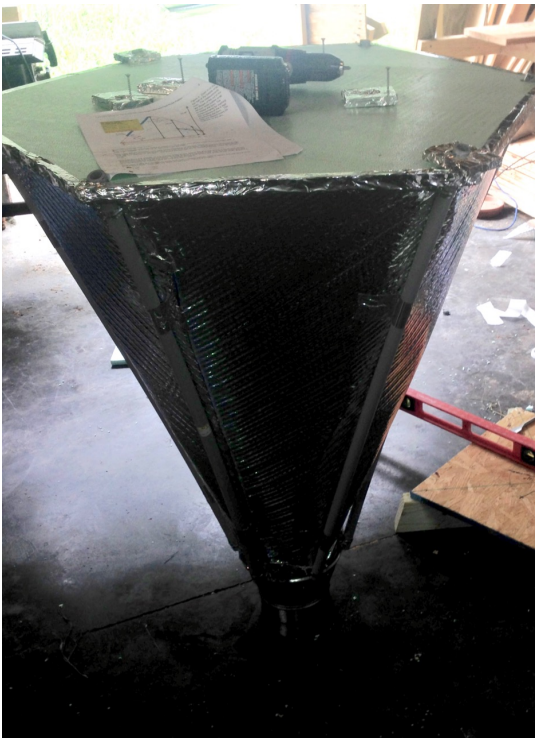
Figure 13: Completed horn! The horn has the lid on top and the pipe reducer on the bottom. Because of the symmetry of the horn, it acts as (tippy) table. The lid connectors are screwed through the lid to small pieces of wood 3 inches from the ends of the legs.
