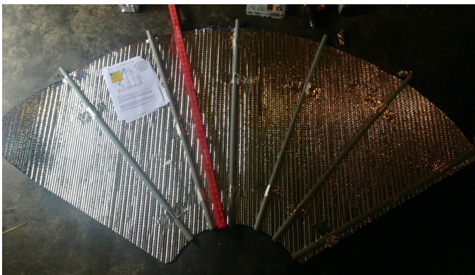
Figure 8: Steps of cutting wrap and attaching pipe legs. The upper left figure shows drawing the inner and outer arcs, the 1.5-2-inch overlap on both sides and measuring and marking the leg positions. Starting with the center pole, add the inner piece of the lid plywood part.
