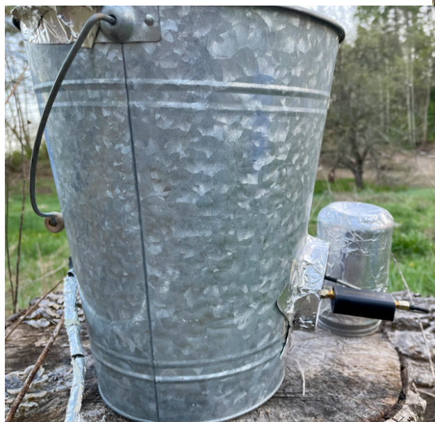
Figure 9: A side view of the Pail with NooElec HI amplifier attached. The weather shielded container is a large empty plastic peanut butter jar. These are great because they are free, unbreakable and metal tape sticks to them well. The lid is taped to the horn, and the jar is covered with metal tape to shield the amplifier from interference from computers and phones.
