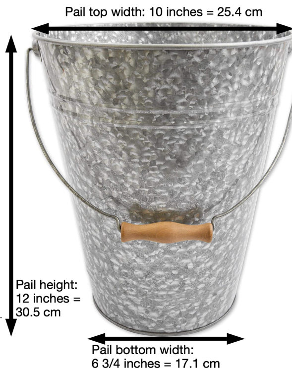
Figure 5: Pail used for our simplest radio telescope. Almost any galvanized pail will do. The bottom should be between 13.5 and 17. cm in diameter. The pail should open up gradually to gather more signal. The pail must be at least 30 cm tall. Bigger is better.
