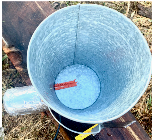
Figure 8: Completed assembly of the horn feed for the radio telescope. The orange ruler at the bottom of the Pail is 8 cm long. The narrow silver wire (4.7cm long) points straight into the center of the pail and is above the bottom of the pail by 7.4 cm.
