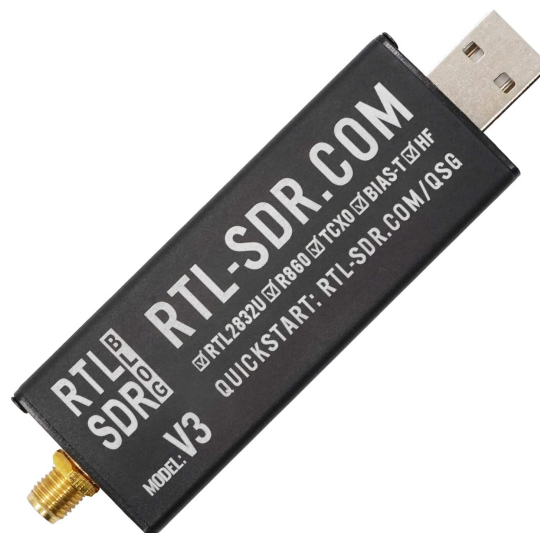
Figure 12: A low cost Software Defined Radio, which has a strong bias-tee and high gain. The down sides to this SDR is that it only has an 8-bit sampler and works well only below 2.4 MHz bandwidth.
