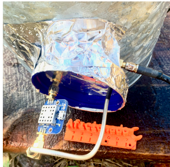
Figure 10: Inside view of the peanut butter jar lid with amplifier and connecting SMA cables. This example shows the GPIO Labs amplifier, which fits in the same place as the NooElec amplifier.
