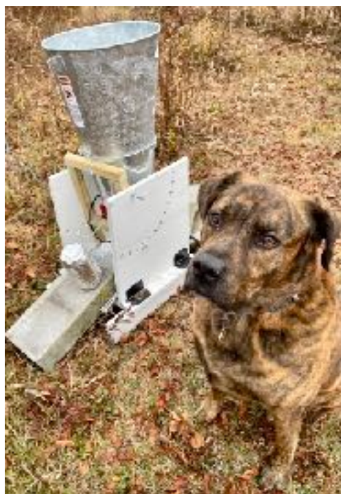
Figure 11: The completed base with pail horn (type B) attached. Note the bolts are used as hinges for the angle reference and a 3rd bolt is used to set the elevation angle. Oni, my dog and mascot, is enjoying the observations.
