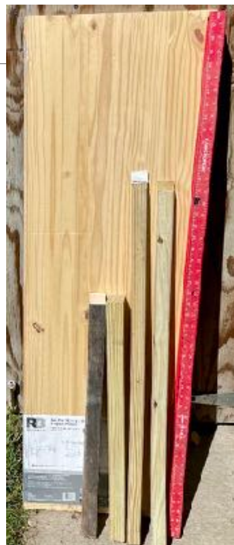
Figure 2: Wooden parts for horn base. The Red 4 foot ruler is for scale. The most expensive part is the 16 by 48 inch shelf, plus two short 2x4s and 2 balusters.
