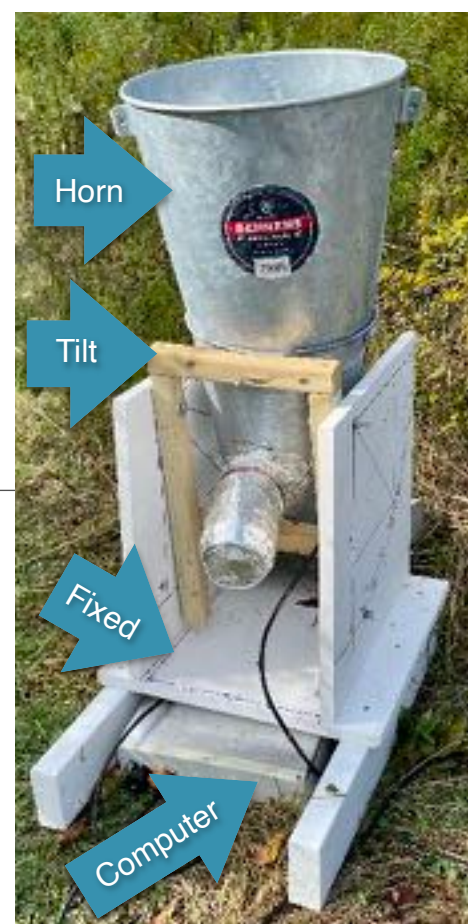
Figure 1: Completed horn radio telescope. The total height of the telescope is about 3 feet (1m). The fixed part is white and the tilting part is brown.
