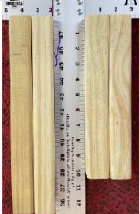
Figure 6: Cut the balusters into two 12 inch pieces and two 10 inch pieces.
