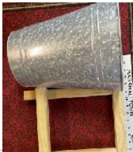
Figure 10: Pail Horn with tilting shelf. The pail will be bolted onto the front and rear pieces
