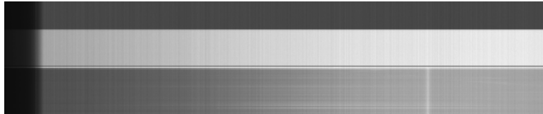
Figure 2.51: Test with LNA open, with 75\Omega load, and antenna attached. Waterfall plot with time on the vertical axis and frequency on the horizontal. Broad horizontal structures only visible in the bottom third section when the antenna is connected.
