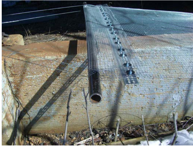
Figure 4.12: The fixed end of the mesh pulling test setup.
