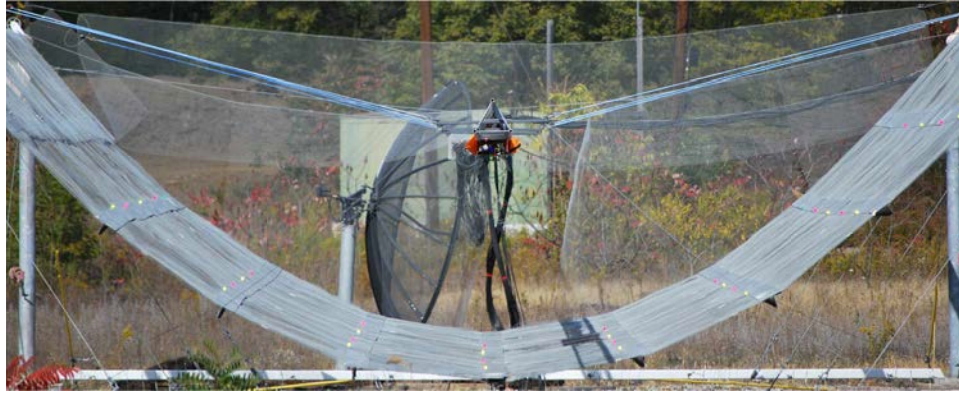
Figure 2.20: West cylinder image used to fit the parabolic cylinder shape. Camera is centered at the feed height.
