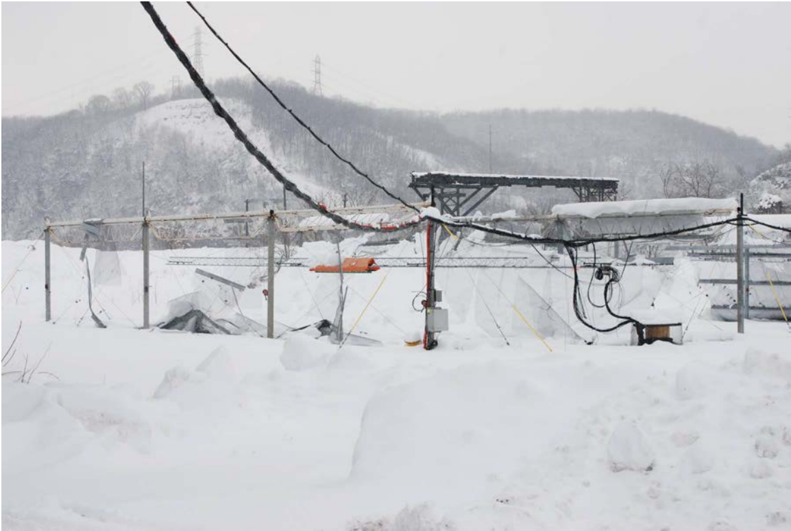
Figure 4.4: After more snowfall and a few days, the East cylinder collapsed fully on the east side.
