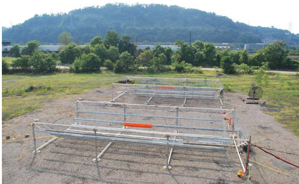
Figure 2.1: The Pittsburgh cylinders viewed from above looking west. Orange covering is the instrumented feed-line. Each cylinder is 10m wide, 25m long, and spaced 25m East-West.
