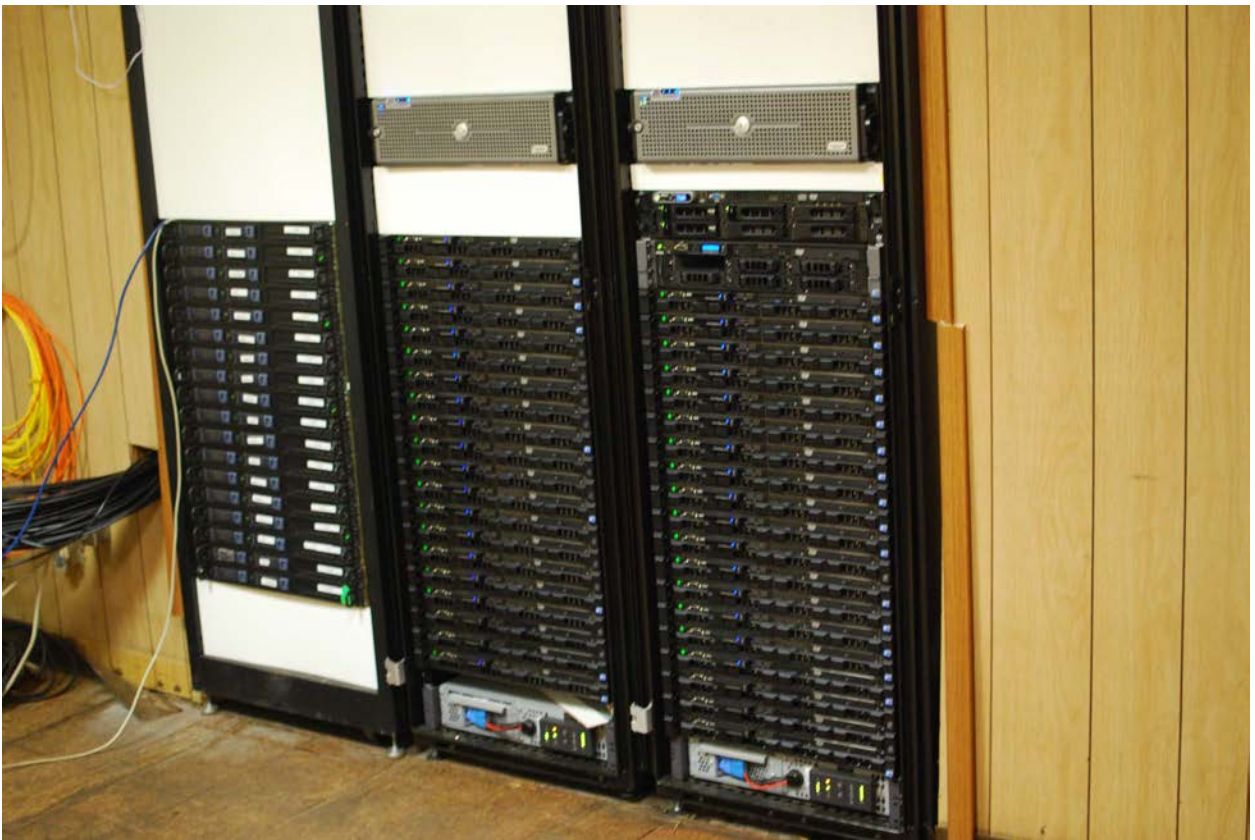
Figure 2.17: The PC cluster of correlator machines. The 16 machines on the far left contain the ADC's. They were used for sampling and FFT. 32 of the dual CPU quad core machines are used for FFT and correlation. The data is stored on the RAID boxes at the top of the image.
