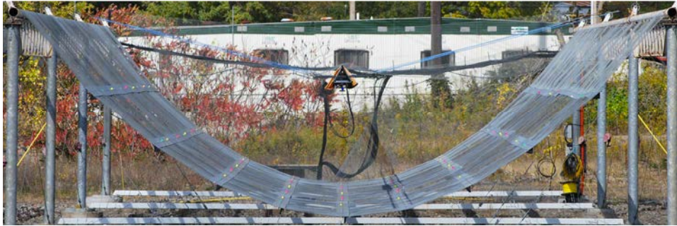
Figure 2.19: East cylinder image used to fit the parabolic cylinder shape. The bottom of each florescent marker is marked with software and then fit to a parabola, assuming a 78 or 77 inch focus depending on the cylinder. The best fit focus is then marked on the image.
