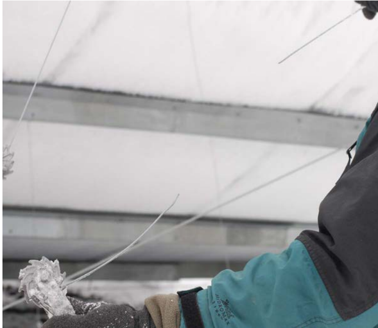
Figure 4.6: The wire was designed to be the failure point. This is an example of a wire that failed as expected.
