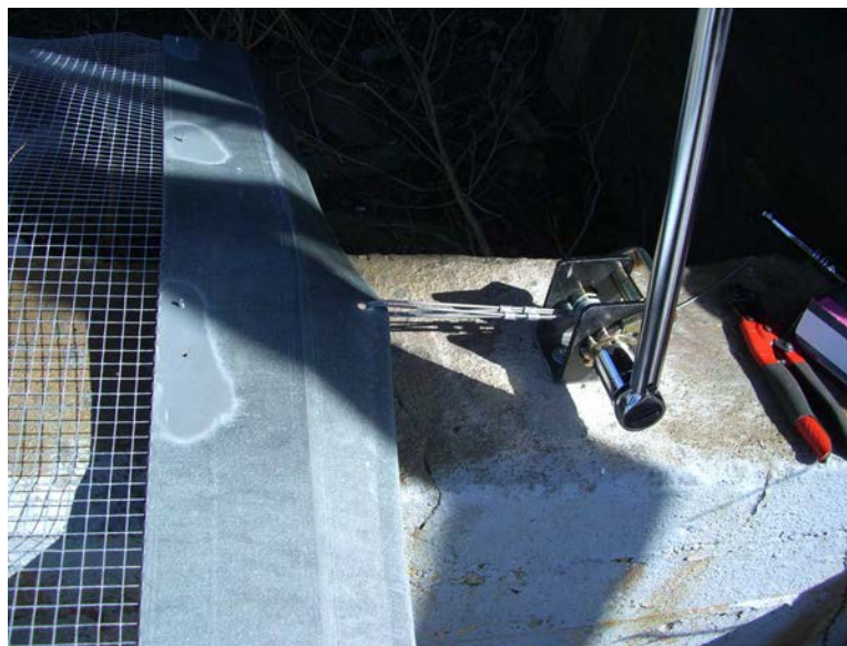
Figure 4.13: Test of mesh connection similar to the as-configured termination. Both wires were pulled straight instead of at an angle. The bend in the finger plate straightened out at 1800 lbs of tension. At 2600 lbs the plate buckled in the perpendicular direction and the wires sheared through the punched hole.
