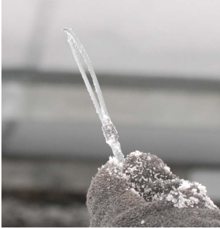
Figure 4.5: The wires were designed to be the failure point. Most wires that broke failed where they were bent to a small radius.
