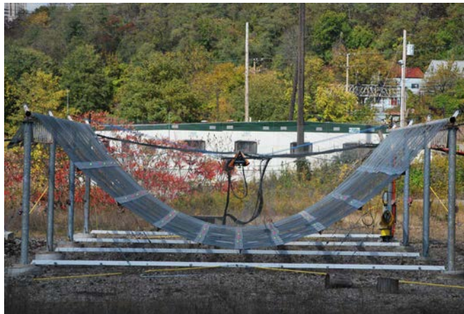
Figure 4.31: East cylinder raised and adjusted, mesh added back along the top side.
