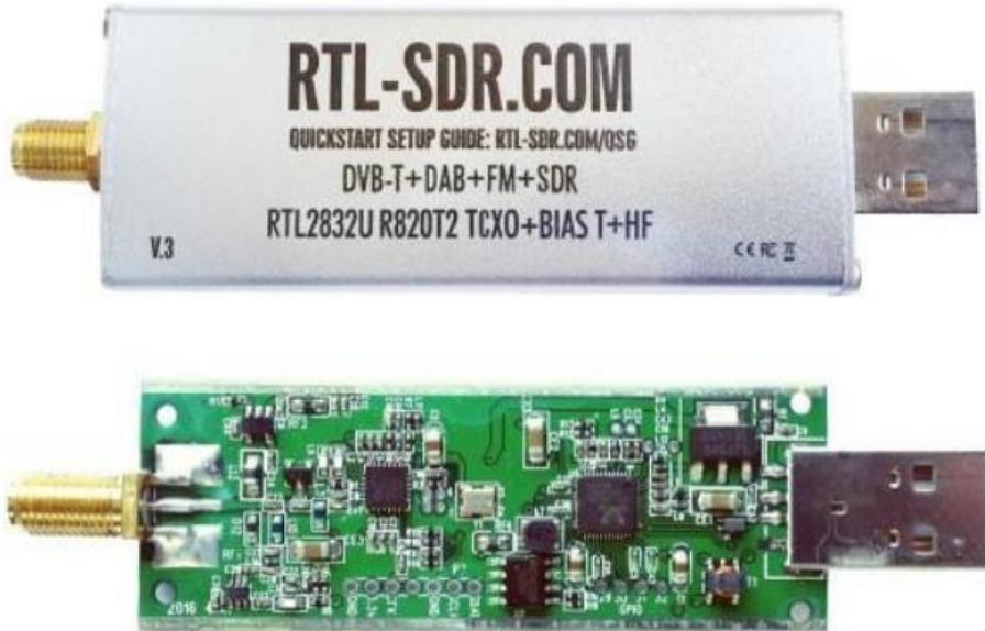
The device that I chose pictured above is the RTL-SDR v3. This device was designed specifically with SDR needs in mind and is cheaper compared to Airspy or the FlightAware dongle. The RTL-SDR v3 has a bandwidth of 2.4 MHz with a frequency range of 500 kHz – 1766MHz. And since it will be used for detecting neutral Hydrogen that frequency range was satisfactory.
